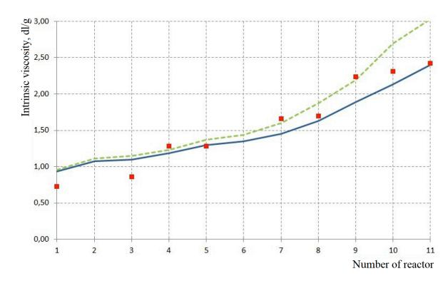
Figure 4. The dependence of the calculated and experimental values of the intrinsic viscosity on the number of the reactor in the cascade (dashed line – simulation results for 15 hours of the process, solid line – simulation results of 30 hours of the process, points – data from the production experiment)
