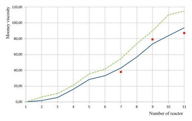
Figure 7. The dependence of the Mooney viscosity of the styrene-butadiene copolymer on the number of the reactor in the cascade (dashed line – simulation results for 15 hours of the process, solid line – simulation results of 30 hours of the process, points – data from the production experiment)
