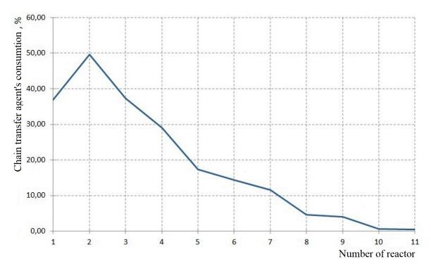
Figure 6. The dependence of the calculated values of the concentration of the chain transfer agent from the number of the reactor
