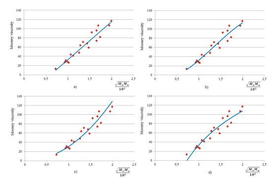
Figure 1. The dependence of the Mooney viscosity on the geometric mean number-average and weight-average molecular weights of the product: a) linear, b) cubic, c) power, d) logarithmic (line – regression dependence, points – experimental data)
