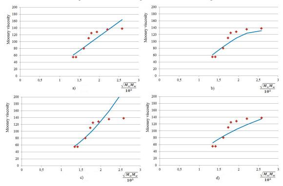
Figure 2. The dependence of the Mooney viscosity on the geometric mean number-average and weight-average molecular weights of the product obtained in the batch reactor: a)
