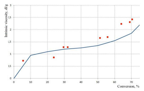
Figure 5. The dependence of the calculated and experimental values of the intrinsic viscosity on the conversion of monomers (dashed line – simulation results for 15 hours of the process, solid line – simulation results of 30 hours of the process, points – data from the production experiment)
